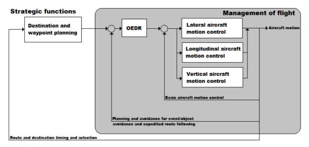
Figure 1. Schematic view of UAS Operation - schematic based on SAE J3016, JUN2018
