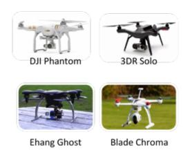
Figure D - 1 - Multi-Rotor UAS with Monocoque Body Construction
