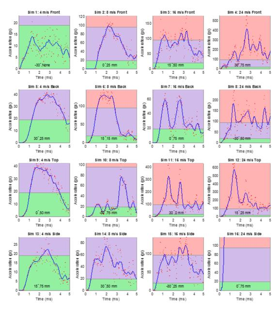
Figure 48 - Acceleration vs Time History for DOE Simulations
