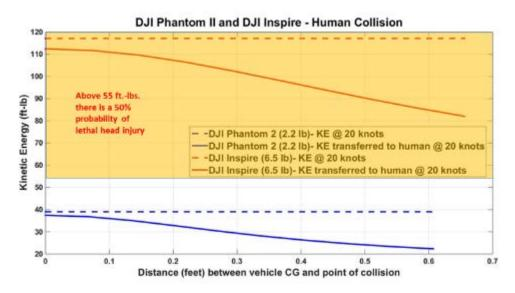
Figure 5 - Low Order Modeling of Impact KE Transfer Based on Vehicle and Body CG Offset
