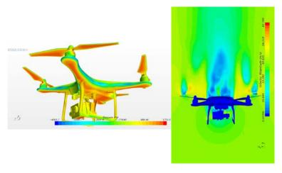
Figure 39 - Images from the Phantom 2 CFD Analysis
