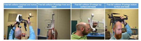
Figure 24 - Potential Collisions between UAVs and a Human Head
