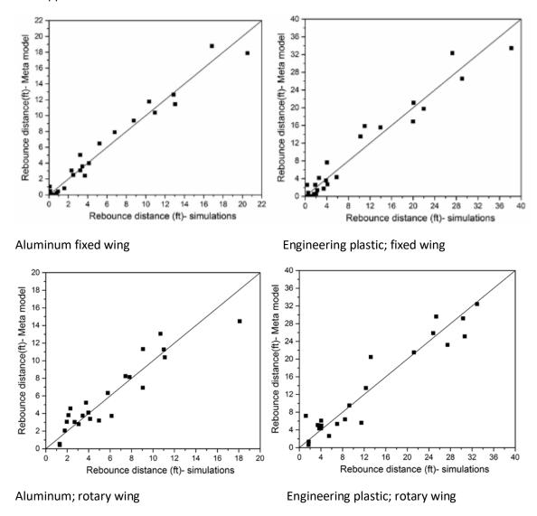
Figure 60 - Comparison of the Rebounce Distance of UAS Predicted by Meta Model and Numerical Simulations
