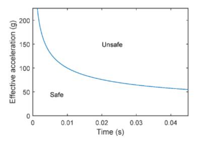
Figure 1 Gadd Severity Index
