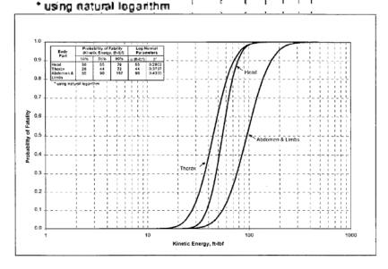
Figure 13 - Probability of Fatality from Debris Impacts for Various Body Parts<sup>76</sup>
