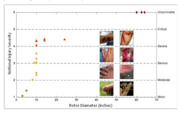
Figure 27 - Notional injury severity index103 vs. rotor diameter for reported incidents104'105'106'107
