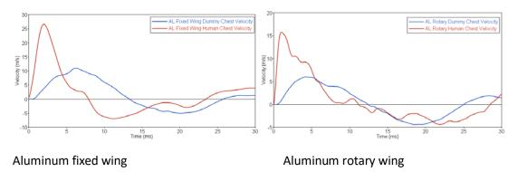
Figure 65 - Comparison of Model predicted Compression Velocity-Time History of ATD and Human Torso under the Impact of UAS ( $\theta$ =90°; V=30 m/s (98.4 ft/s))
