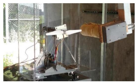
Figure 28 – Laceration Testing Setup
