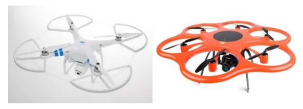
Figure D - 11 - Propeller Guards (left); Shrouded Propellers (right)
