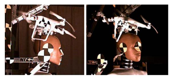
Figure 45 - Phantom 3 Standard Fuselage Deformation During NIAR 50-foot Drop Test Impacts (Test UA17A-13)
