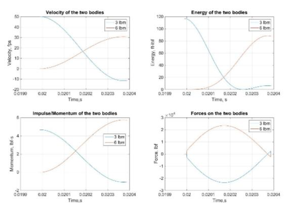
Figure 3 - Model Outputs Detailing the Collision of a 3 lbs Object with a 6 lbs Object
