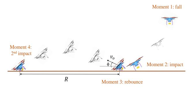
Figure 58 - UAS Collision on the Ground and Rebounce
