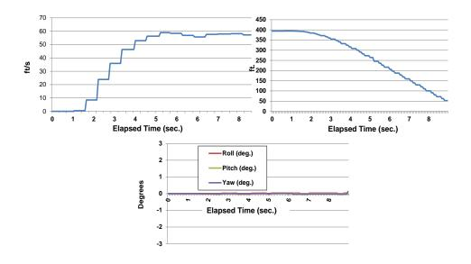
Figure 41 - Phantom 2 Limited Flight Test Telemetry Data; Rate of Descent vs. Time (upper left),
