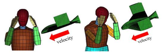
Figure 70 - Impact Modeling with Guarding and Bracing Postures
