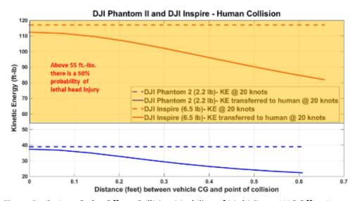
Figure D - 8 - Low Order Off-set Collision Modeling of Multi-Rotor UAS Offset Impact
