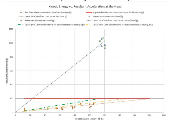
Figure 23 - Resultant Force versus Impact KE for Steel, Wood and Phantom 3
