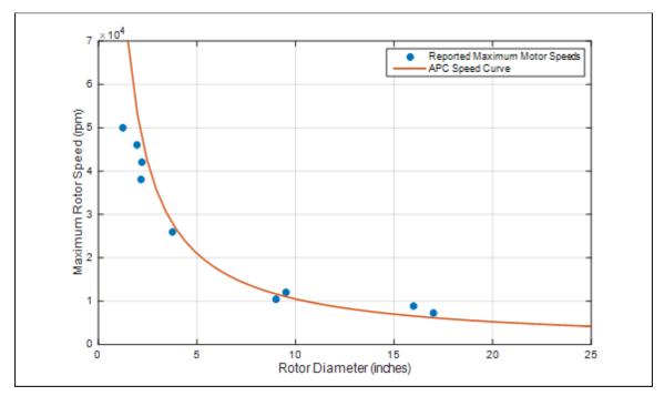
Figure 25 - Rotor Speed vs. Rotor Diameter for Multi-Rotor UAS, Compared with APC RPM Curve
