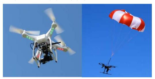
Figure D - 25 - Visual Warning Systems on Multirotor UAS (left); Parachutes on Multirotor UAS (right)
