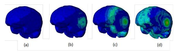
Figure 51 - Stress Wave (von Mises) Propagation through the Brain at Times (a) 0, (b) 0.19, (c) 0.5, and (d) 0.813 ms
