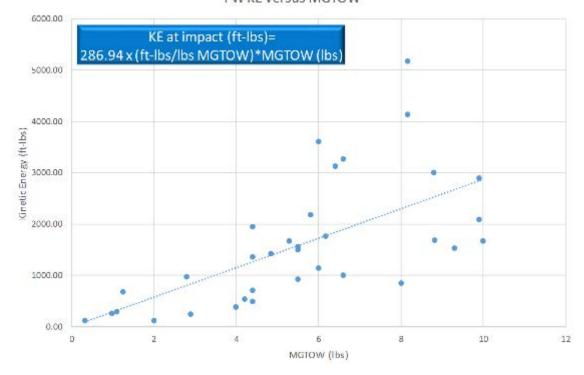
Figure 43 - Relation of MGTOW to KE at Terminal Velocity for Fixed Wing UAS < 10 lbs
