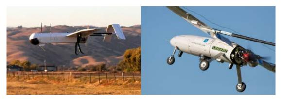
Figure D - 20 - Fixed Wing UAS with Skid Landing Gear (left); Standard Landing Gear (right)
