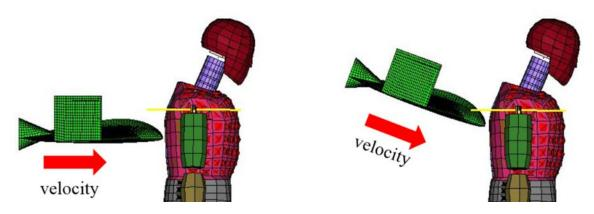
Figure 72 - Posterior UAS Impact Modeling
