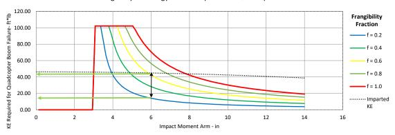
Figure 67 - Kinetic Energy Needed for Failure of Quadcopter Boom Compared with Kinetic Energy Transferred Based on Theoretical Flight Condition  $u_1=50\ ft/s$
