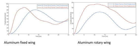
Figure 64 - Comparison of Model-Predicted Displacement-Time History of ATD and Human Torso under the Impact of UAS ( $\theta$ =90°; V=30 m/s (98.4 ft/s))
