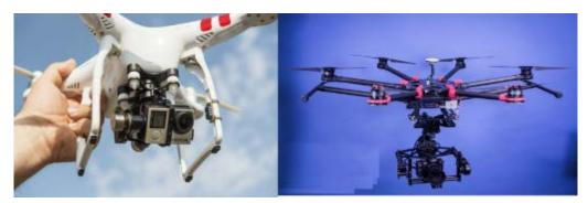
Figure D - 22 - Small Gimbals and Camera (left); Large Gimbals and Cameras (right)
