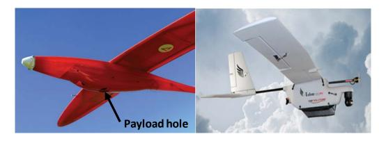
Figure D - 24 - Payload inside the Fuselage (left); Payload Protruding Outside the Fuselage (right) Helicopter-Style RW UAS:
