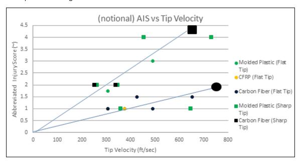
Figure 30 – Injury Severity vs. Tip Velocity
