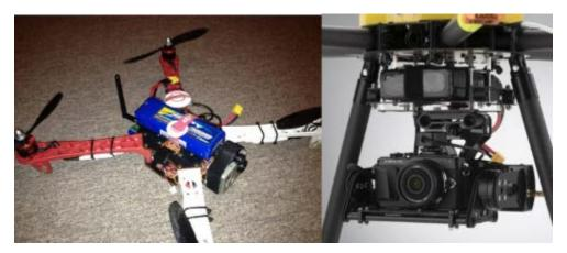
Figure D - 14 - Battery Mounted above Main Body with Velcro (left); Battery Mounted Below Main Body (right)
