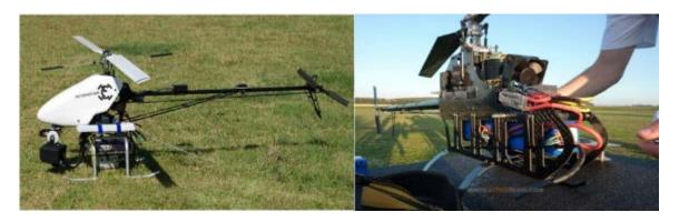
Figure D - 17 - Batteries on Side of Fuselage (left); Batteries inside the Fuselage Belly (right)
