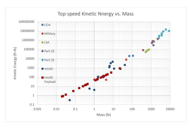
Figure 8 - Estimated Terminal KE for UAS and Manned Aircraft  $^{69,70}\,$
