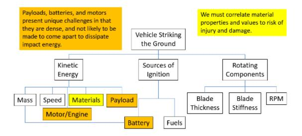
Figure 2 - Ground Collision Severity Taxonomy Defined for the A4 Task
