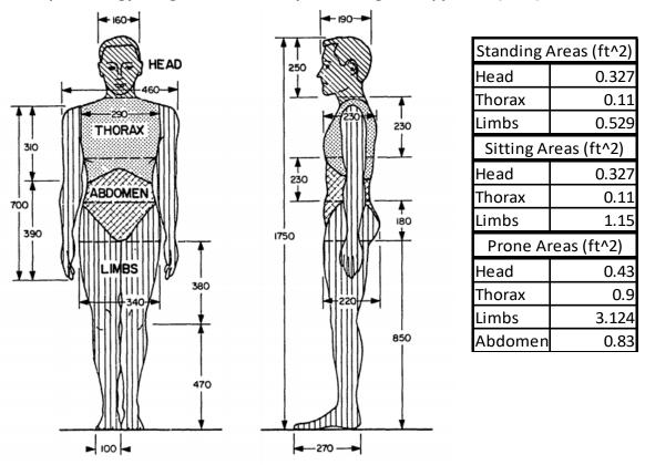
Figure 16 - Janser Standard Man Dimensions and Calculated Projected Areas<sup>19</sup>
