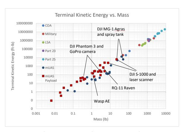
Figure 7 - Comparison of Estimated Kinetic Energy for Several Manned Aircraft, UAS and UAS Payloads
