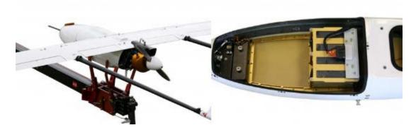
Figure D - 16 - Rear-Mounted Engine on a 50 lbs UAS (left); LiPo Batteries inside the Fuselage of a 33 lbs UAS (right)
