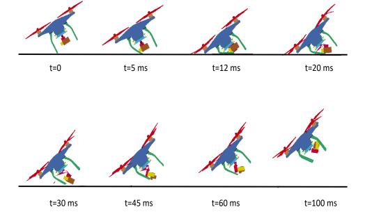
Figure 59 - Model Predicted Rebounce Behavior of a Rotary Wing UAS (Phantom 3) Collision on the Ground (V=32.8 ft/s;  $\theta$ =60°)
