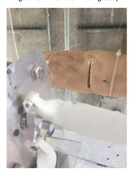
Figure 29 – Example of Deep Laceration from Propeller Strike
