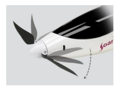
Figure D - 12 - Folding Propellers
