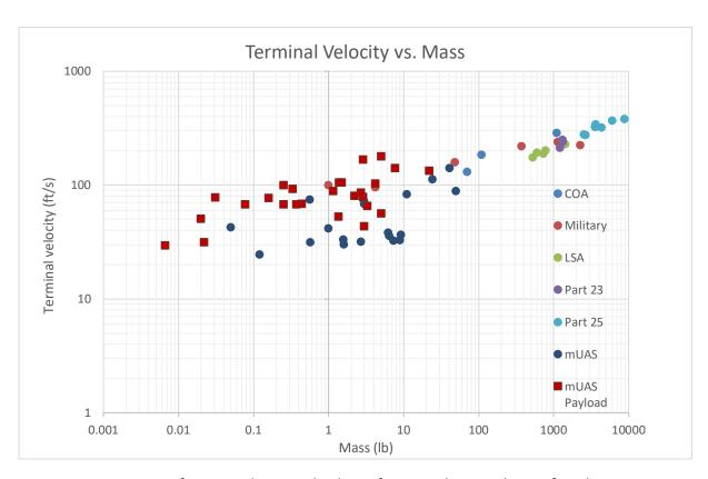
Figure 6 - Comparison of Estimated Terminal Velocity for Several Manned Aircraft and UAS Departing Controlled Flight from 400 ft AGL 69'70
