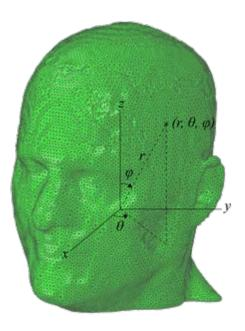
Figure 47 - Spherical Coordinate System for Head Impact Simulations
