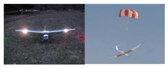
D-Figure D - 26 - Fixed Wing UAS with Landing and Position Lights (left) and Parachutes (right)
