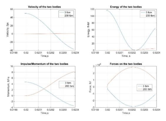
Figure 4 -Model Outputs Detailing a Collision Between a 3 lbs Object and a 200 lbs Object
