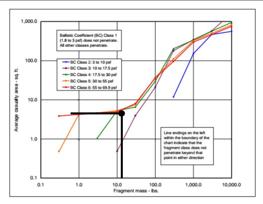
Figure 38 - Penetration Effects on Type A Roof Structure (per Table 40 definition of roofing types)<sup>114</sup>
