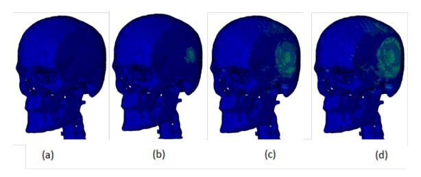
Figure 50 - Stress Wave (von Mises) Propagation through the Skull at Times (a) 0, (b) 0.375, (c) 1, and (d) 1.275 ms
