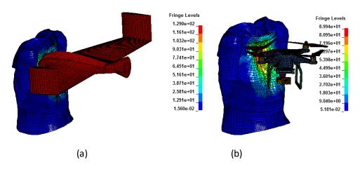
Figure 63 - Model Simulated Typical Deformation Response of Human Torso under the Impact of UAS ( $\theta$ =90°; V=30 m/s (98.4 ft/s)): (a) Aluminum Fixed Wing; (b) Aluminum Rotary Wing
