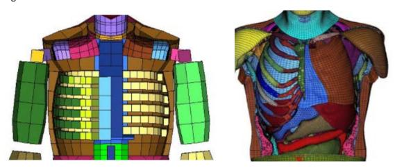
Figure 61 - ATD Torso Model (left) and Human Torso Model (right)
